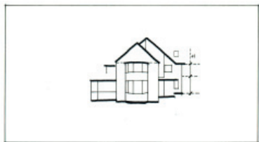
Eave height analysis of the proposed No 11 Luard Road and the adjacent properties
