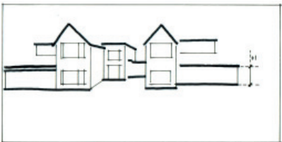
Eave height analysis of the proposed No 11 Luard Road and the adjacent properties
